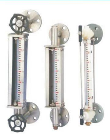
Gauge is fitted between two end blocks through gland packing. The Gauge is mounted parallel to tank so as to form a close loop causing tank liquid to seek its level in gauge. Guards are provided in the form of tie-rods / C-channels around the gauges to protect it from accidental blows. End blocks have built-in isolating valve, Drain Valve & vent plug.
