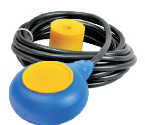
LSC is simple and reliable switch for level detection. It can be used for small or long range of storage tanks and reservoirs. Polypropylene rigid construction provides prevention from corrosion. Float tilt with liquid in rise & fall condition, accordingly micro switch operates from NO (Normally Open) to NC (Normally Close) position. It can be used as a multipoint switch also.
